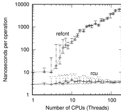
**Figure 9.28:** Performance of Preemptible RCU vs. Reference Counting
