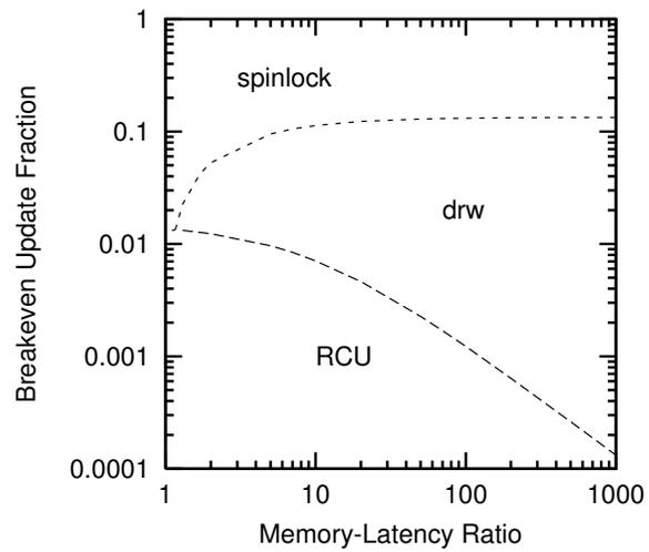
**Figure 17.7:** Breakevens vs.  $r$ ,  $\lambda$  Small, Four CPUs
