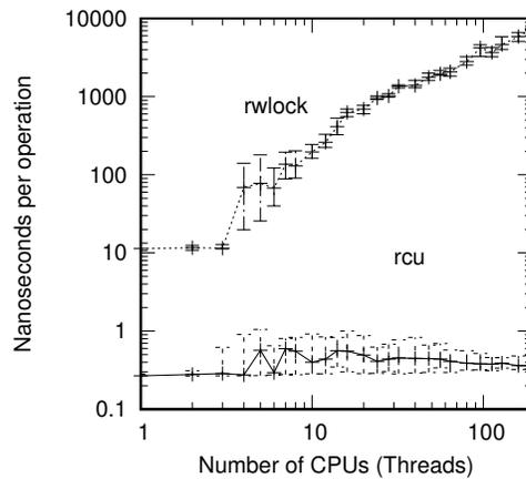
**Figure 9.23:** Performance Advantage of RCU Over Reader-Writer Locking
