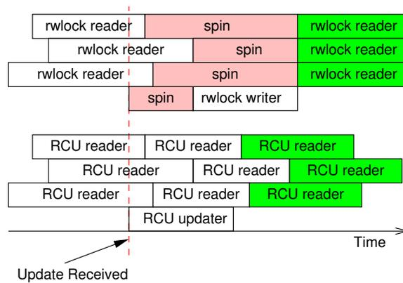
**Figure 9.26:** Response Time of RCU vs. Reader-Writer Locking
