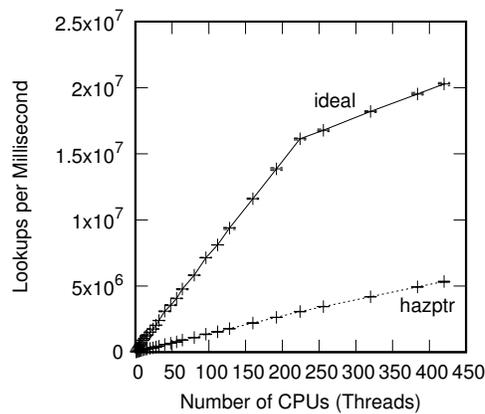
**Figure 9.3:** Pre-BSD Routing Table Protected by Hazard Pointers
