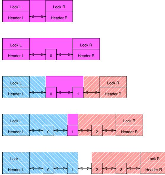
Figure 5.5: Double-Ended Queue With Left- and Right-Hand Locks
