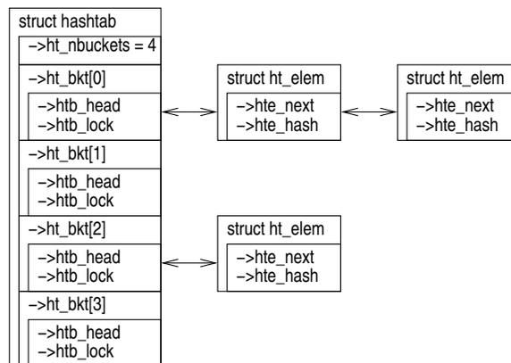
Figure 9.2: Hash-Table Data-Structure Diagram
