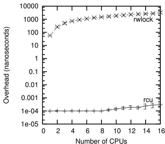
Figure 8.23: Performance Advantage of RCU Over Reader-Writer Locking
