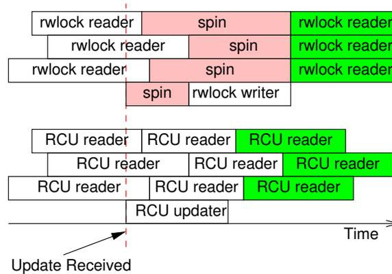
Figure 8.26: Response Time of RCU vs. Reader-Writer Locking
