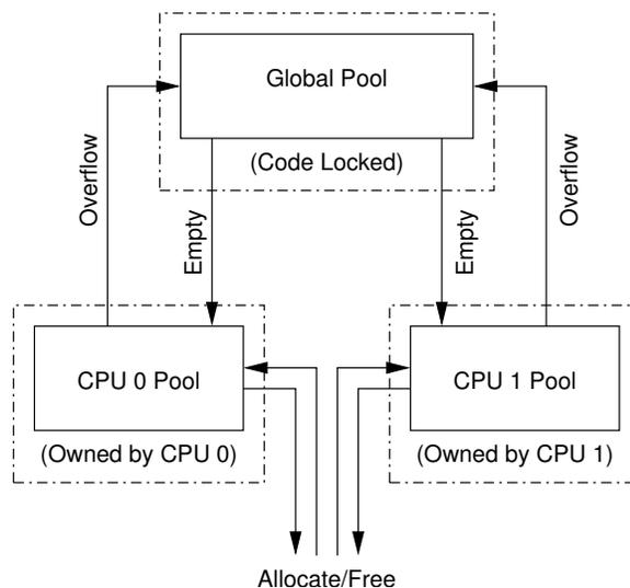
Figure 5.27: Allocator Cache Schematic
