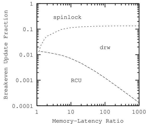
Figure 15.7: Breakevens vs.  $r$ ,  $\lambda$  Small, Four CPUs
