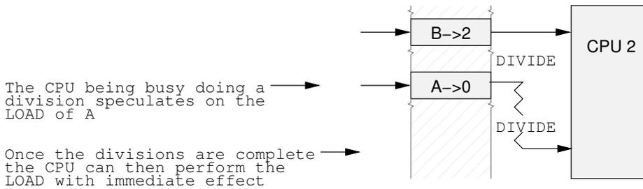
Figure 13.14: Speculative Load
